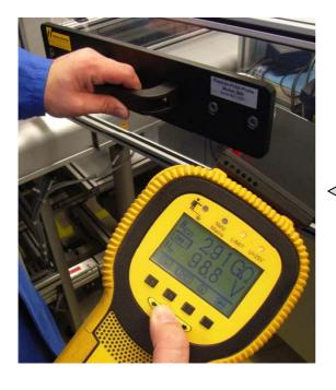
Point to Point R<sub>p-p</sub> machine hood testing
